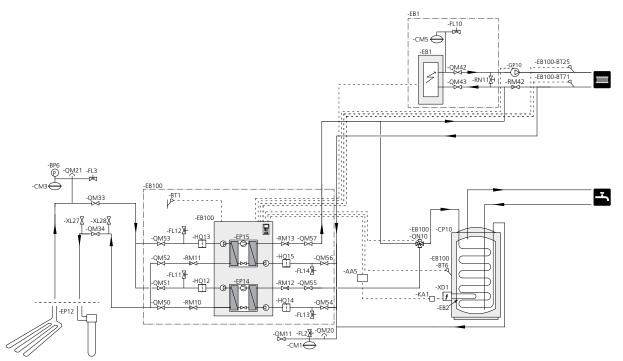
Module EP14 prioritises hot water charging via a reversing valve. When the hot water heater/accumulator tank is fully charged, the reversing valve switches to the heating circuit. The heat pump is controlled by an outdoor sensor combined with the flow line sensor which must be placed on the main pipe to the radiators. ELK 42 is connected automatically when the energy requirement exceeds the heat pump capacity.
