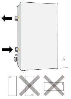
The immersion heater must be installed standing (see image above). An area of 500 mm is required in front of the immersion heater for service work. If this is not possible, detachable connections should be used.
